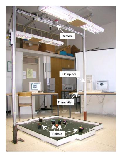
Fig. 1 - The robot-soccer system
